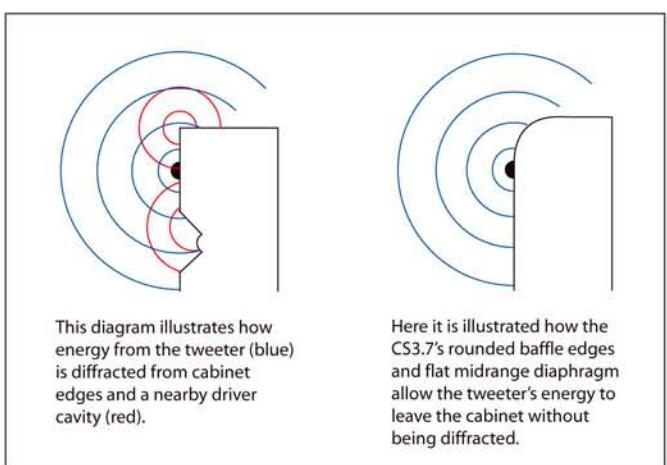
This diagram illustrates how energy from the tweeter (blue) is diffracted from cabinet edges and a nearby driver cavity (red).
