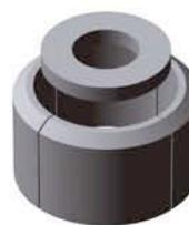
A set of four radially- and one axially-magnetized neodymium magnets have a total weight of 64 grams (2.3 oz), six times usual.
