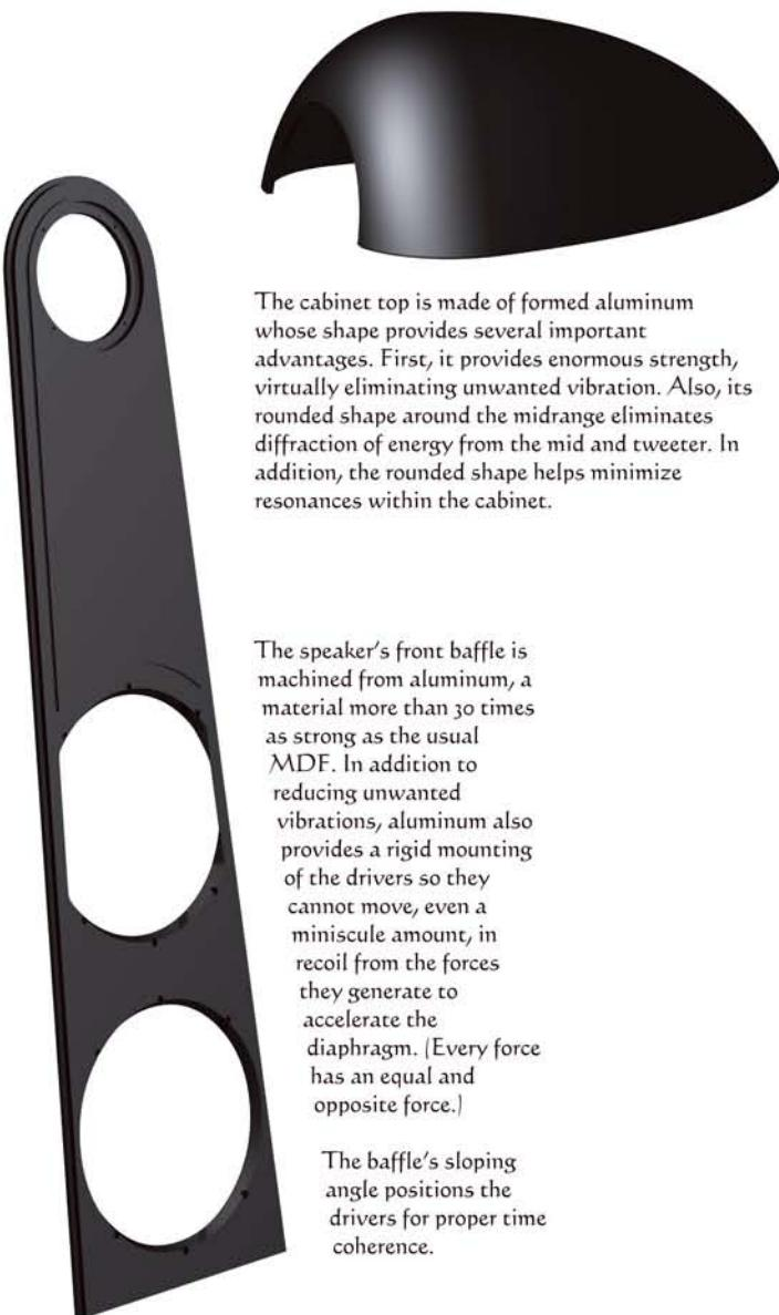
The cabinet top is made of formed aluminum whose shape provides several important advantages. First, it provides enormous strength, virtually eliminating unwanted vibration. Also, its rounded shape around the midrange eliminates diffraction of energy from the mid and tweeter. In addition, the rounded shape helps minimize resonances within the cabinet.
