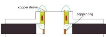
In THIEL's long gap design the shorter coil remains within a long uniform field as it moves through its entire range, drastically lowering distortion.
