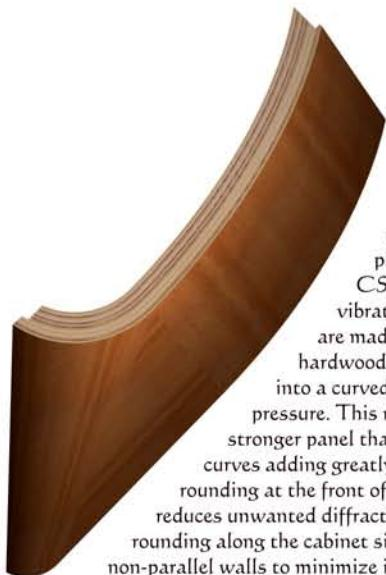
The construction of the cabinet sides also plays its part in the CS3.7's rigid, low vibration cabinet. The sides are made of 15 layers of hardwood laminated together into a curved shape under high pressure. This results in a much stronger panel than usual, with the curves adding greatly to its rigidity. The rounding at the front of the speaker also reduces unwanted diffraction and the gentle rounding along the cabinet sides also creates non-parallel walls to minimize internal resonances.
