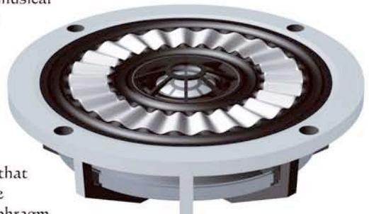
This new diaphragm geometry also has a second important benefit that derives from its shape. The diaphragm is basically flat and therefore has virtually no detrimental effect on the tweeter's output, unlike a normal cone shaped diaphragm that alters the sound of a tweeter mounted in its center.
