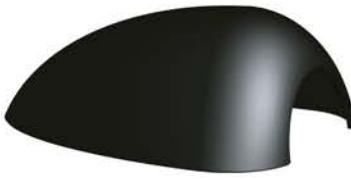
The cabinet "head" is made of formed aluminum into a shape that provides dramatically improved vibration reduction, the practical elimination of diffracted driver energy and the reduction of internal standing waves. Less vibration contributes to greater clarity, while the absence of diffraction allows for very open, boxless reproduction.
