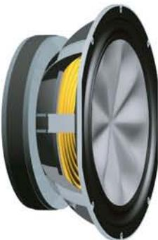
The woofer's diaphragm contributes to extended bandwidth and high efficiency while its very large magnet powers the copper stabilized, long gap motor that achieves distortion levels only one-tenth usual. The result is tonal, effortless, and solid low frequencies.
