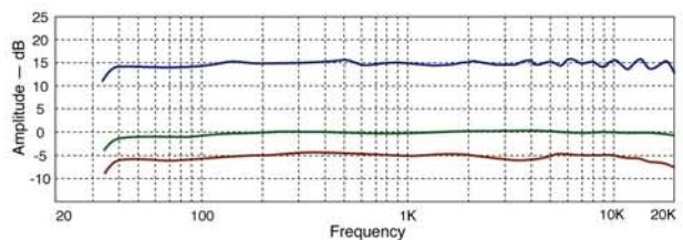
The blue graph is the on-axis anechoic frequency response.
